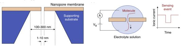
The passage of the molecule through the pore yields information about its structure and chemical properties. Atomically thin two-dimensional materials with nanometer-sized pores, such as single-layer  $MoS_2$ , represent the ideal sensor because of their ultimate thinness. Despite the benefits they offer, their application for peptide sequencing remains challenging since the fast translocation speed provides short observation time per single molecule.
